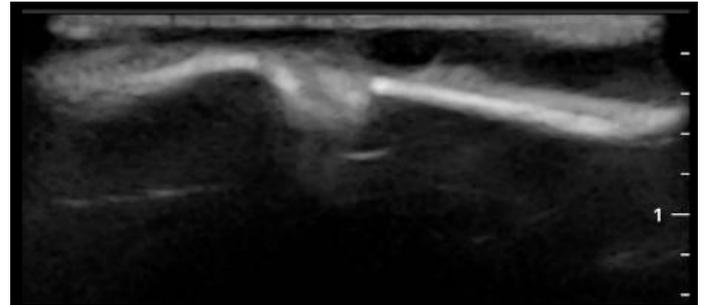
Figure 5: Ultrasound image of the distal/middle phalanx phantom using Butterfly iQ.
