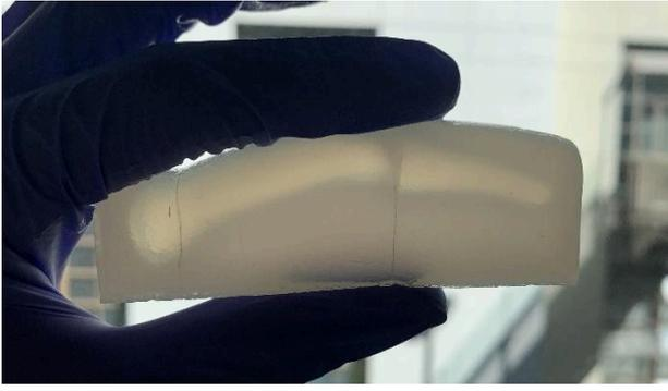
Fig. 3: Phantom of the distal/middle phalanx with 1 mm growth plates.
