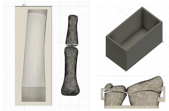
Figure 1: 3-D models of the distal/middle phalanx phantom and casing (left) and radius/ulna phantom and casing(right)
