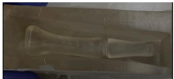
Figure 2: Distal/middle phalanx phantom held up by thin wires before the molding process.
