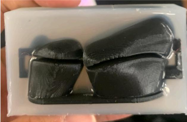
Figure 4: Phantom of the growth plate at the radius and ulna with 2 mm growth plates.
